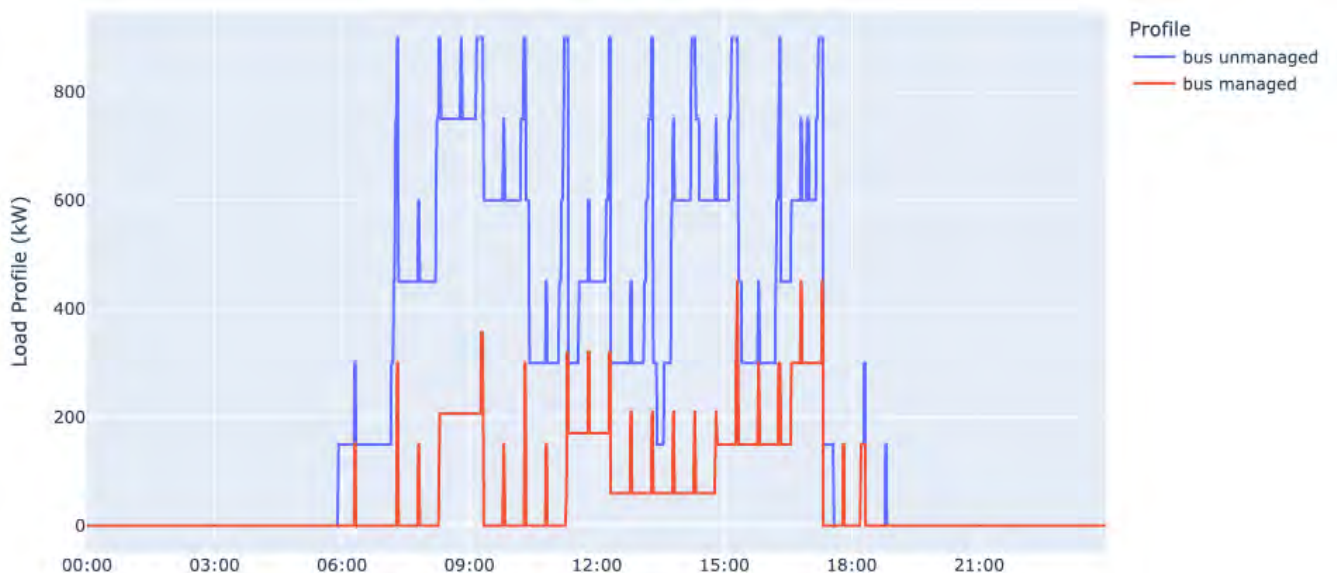
FIGURE 28. CHARGING LOAD PROFILE FOR BUSES AT DRTC
