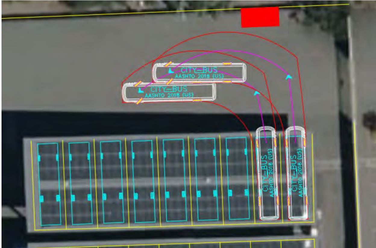
FIGURE G5: VEHICLE TURNING PATH ANALYSIS FOR SOUTH CANOPY STALLS
